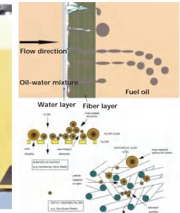
Large-capacity multistage filter principle
