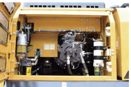
Large-capacity multi-stage filter system
