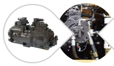
Kawasaki 160CC dual-ratio positive-flow main pump takes full advantage of the flow and realizes demand equal to supply. As compared with negative flow system, it reduces the loss of neutral-position return, and meanwhile response speed is higher and capacity loss is reduced
