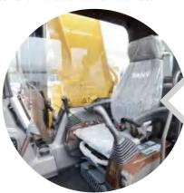
FOPS/ROPS cab is used. Through finite element modal analysis, steel structure and sealing performance of the cab are optimized; its strength is 5 times of general cab, the safety performance is extremely high and meanwhile the cab noise is reduced by 3-5dB, which makes the operation more comfortable.
